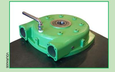
It is also important at this point to attach the filler tube to the back of the pump as it could be difficult to attach once the Geared Motor Unit (GMU) is in place. Line the thread of the breather tube with PTFE tape and tighten into position to give a leak free seal.
