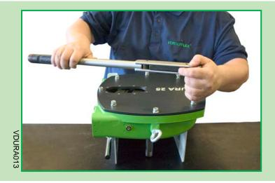
Fit the rest of the cap head screws with washers and torque-tighten.
