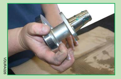
With the hose in position the tapered flanges can be fitted. Apply some pump lubricant to the taper flanges to aid fitment.
