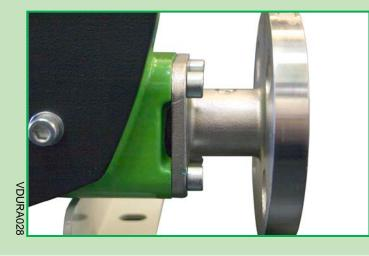
The tapered flange should be pulled toward the housing for as close as is possible ensuring 5mm (16") of the hose can be seen in the gap between the fixing holes.
