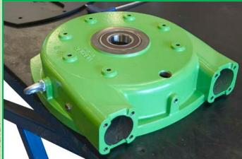
Fit the lifting eye to the case.
