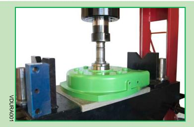
Using a bearing press, press the bearings squarely into the front and rear of the pump body until they locate on the shoulders in the pump housing.
