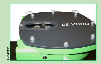
Fit the inspection window gasket to the front cover.
