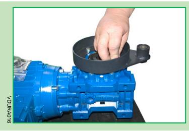
Press fit the torque arm bush into the torque arm; then fasten the torque arm to the GMU with the shaft sleeve facing away from the gearbox before attempting to fit it onto the drive shaft.
