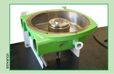
Press the drive shaft through the bearing assembly.
