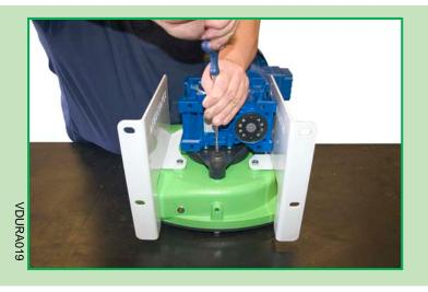
Fasten the torque arm to the housing and complete the installation of the GMU.
