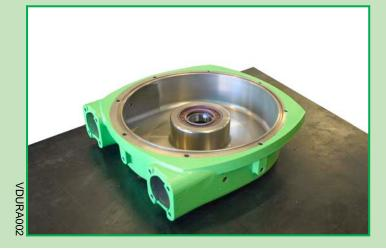
The shaft seal should be pressed squarely on top of the inner bearing with the sprung lip facing into the pump cavity.
