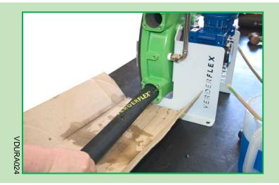
Insert one end of the hose into the mouth of the suction port (the hose should be fed into the pump in the direction of normal operation). Once the hose reaches the rotor, the drive can be inched forward slowly to feed in the remainder of the hose into the pump housing.
