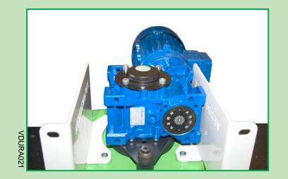
To complete the assembly, mount the dust cover using the screw cap head screws supplied.
