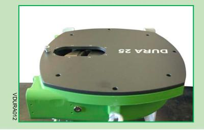
When fitting the front cover, the cap head screw nearest to the inspection window, is fitted without a washer (pictured).
