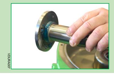
Apply some triple life bearing grease (Roccol Sapphire 2) to the drive shaft before assembly.
