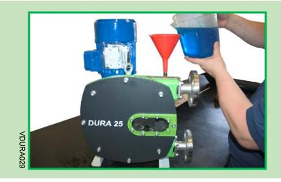
The pump must always be filled with the correct amount of lubricant. Fill to the mid level of the front cover. Check the compatibility of the lubricant with the product being pumped; it can react when mixed with certain types of nitrogenous or oxidizing substances such as nitric acid.
