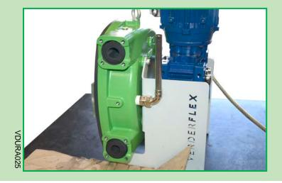
The hose should be inched forward until there is sufficient hose protruding from the suction and discharge ports to fit the tapered flanges (10mm). If the hose passes this point the drive should be reversed and inched back slowly into the correct position.
