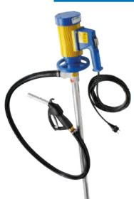
**Electric universal motor JP-280,** 230 V, 50/60 Hz, 825 W internally ventilated motor, splash protection to IP 24, on/off switch, 5 m cable with plug, double isolated class II, over load protection switch with low voltage release
