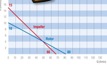
$\label{eq:JP-SS-41-1.000} \text{JP-AIR2, JP-SS-41-1.000, test media water 20 °C, pressure pipe 1", oval gear meter, measured values: $\pm 5\%$ and $\pm 5\%$ are the pipe 1".}$
